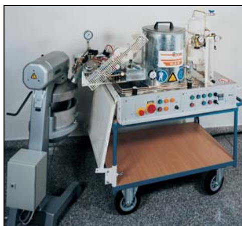
Figure 4: Example of a laboratory scale foamed bitumen unit
