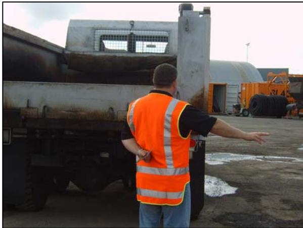
Figure 5b: The incorrect placement of a Spotter at the rear of the vehicle. As the mirror is out of sight of the Spotter, the driver does not have a clear view of them.
