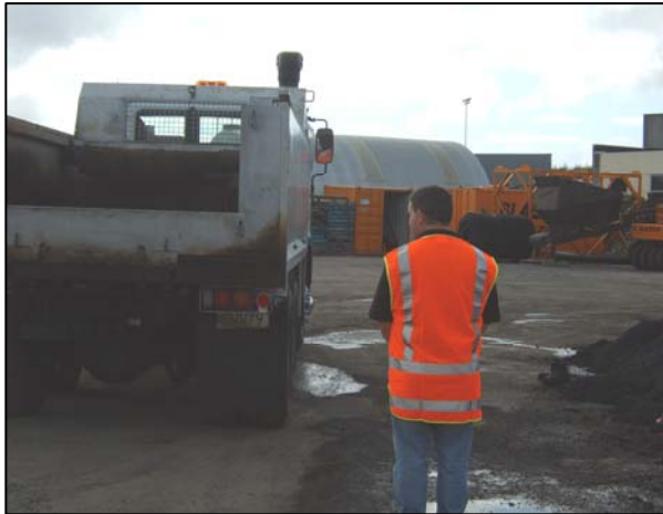
Figure 5a: The correct placement of a Spotter at the rear of the vehicle. A clear view of the Spotter is seen in the driver's mirror.
